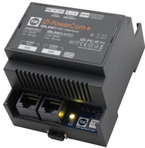
The **IZI-PowerCom+** is an **IZI-Link+ PowerLine communication interface** module that **sends and receives lighting control data and statuses over a low-voltage 2-wire power line**, allowing you to control, monitor and configure IZI-Link+ compatible products.
