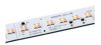
The MTW4270 is a tunable white LED module that is capable of changing its colour temperature from 4000K to 2400K. This allows the user to create a dynamic ambience with the extra warm 2400K colour temperature as a unique feature.
