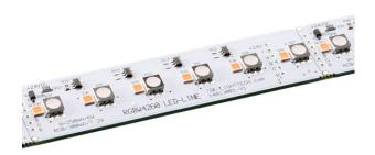
The RGBW4260 is a multi-purpose LED module combining RGB with Tunable White technology. Its RGB function allows the user to create playful and vibrant colour effects. While its Tunable White technology offers mood control by varying colour temperature between neutral white (4000K) to very warm white (1400K). This offers unprecedented freedom in lighting design with one single LED module.
