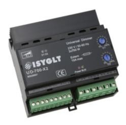
The AD-UD700 is a universal dimmer that is suitable for highvoltage luminairs and LED retrofit lamps. Two independently controllable outputs which have a 700W output each. Parrellel connection is possible creating a combined 1400W.
